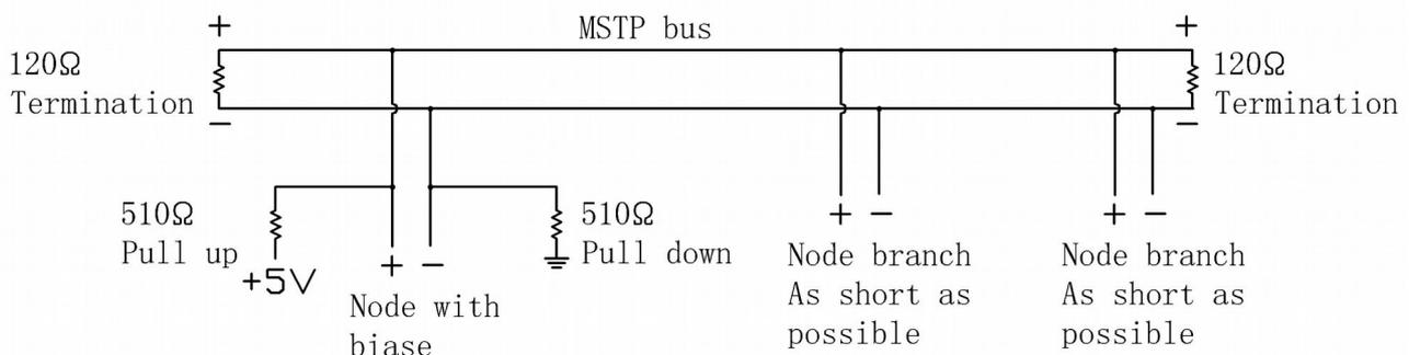
Figure: MSTP bus showing termination/bias resistors
